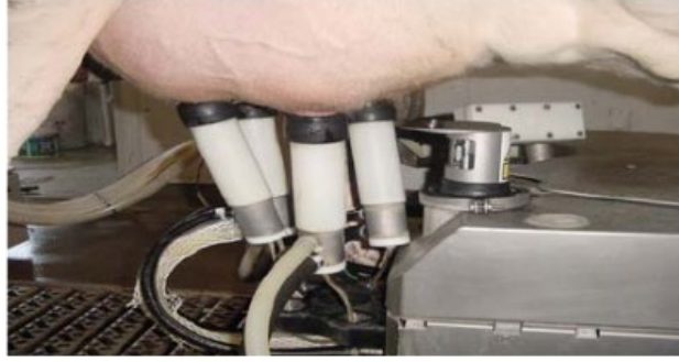
Figure 3. Milking process in robotic milking system
